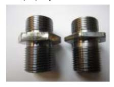
The problem is solved by modifying the hex section of the union bolt, making it thinner to allow clearance for the filet to screw on further and properly compress the rubber seal ring.
