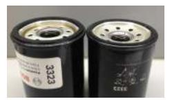
The Problem: Filter manufacturers have changed the design of their oil filters so they are no longer compatible with the union bolt fitting on the FJR. The old style filter with a concave end is on the right, the new style with convex end is on the left.
