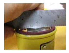
Placing a straight edge across the convex filter shows the problem. The filter base bottoms on the hex before it can screw on enough to compress the rubber sealing ring.
