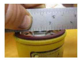
Placing a straight edge across the convex filter with the modified union bolt shows the needed clearance restored. Filter can now be torqued to properly compress the rubber
